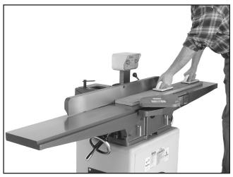
**Figure 28.** Typical surface planing operation.
